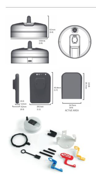
Dimensions in millimeters (dimensions in inches)
