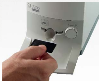
Unit detects if plates are inserted upside down.
